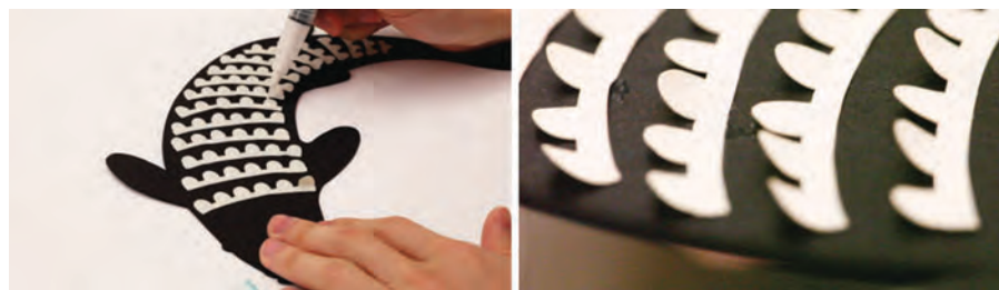
FIG. 5. Living paint. Spore solution as an active ink to actuate toy fish scales. Color images available online at www.liebertpub.com/3dp
