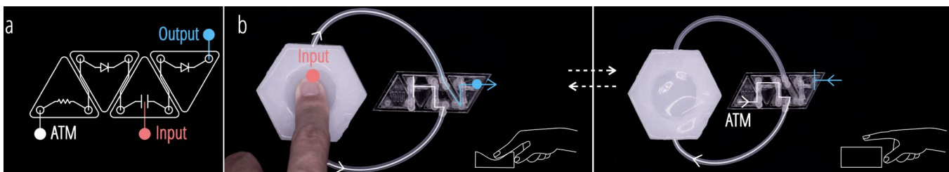
Figure 10: The fluidic filter. a) Design diagram of the capacitor. b) (Left) When the capacitor is squeezed by the input, the left diode is blocked and the airflow is released from the right diode; (Right) When the capacitor is rebounded, the left side diode is fed and the right side diode is blocked.
