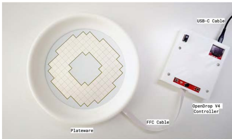
Figure 6: A complete Dancing Delicacies system consists of a plateware with an embedded electrode board connected to an OpenDrop V4 controller via an FFC cable, and a USB-C cable for communication and powering.
