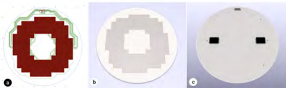
Figure 4: a) A printed circuit board holds the electrode array; b-c) The individual electrodes are connected to the backside of the circuit board through vertical interconnects and linked to a connector on the back with 128 channels.
