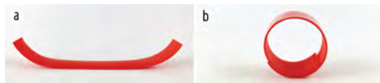
Figure 4: Bending actuator at neck brace scale (15cm x 1.5cm) using: (a) PLA 0.5mm actuator and 0.5mm constrain layer (b) PLA 1mm actuator taped to PET film, each triggered in an oven at 75oC for 1 min.
