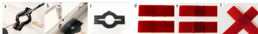
Figure 13: (a) Spread MWCNTs-PBS on the PET. (b) Use a film applicator to make a thin film. (c) Cured MWCNTs-PBS after 12 hours in the oven. (d) PLA with printed mesh. (e) Applied Thinking Putty. (f) Two healed pieces.
