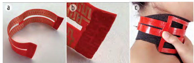
Figure 6: (a-b) Thinking Putty applied to each module’s edges. (c) Self-fusing edges connect modules.
