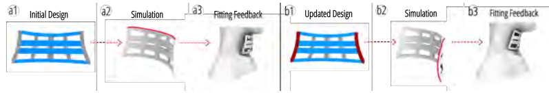
Figure 11: (a1) Initial design (a2-a3) Visual simulation feedback for bending and fit (b1) Designer updates design with two actuated curves on the sides (b1-b3) Simulation shows the updated design fits better.
