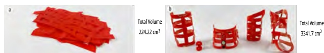
Figure 17: (a) Total volume of flat artifacts is 224.22 \text{ cm}^3 (b) Total volume of artifacts after assembly is 3314.7 \text{ cm}^3 .
