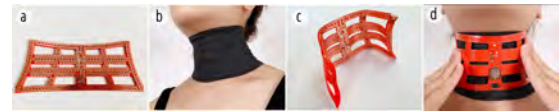
Figure 2: (a) Initial flat state of ExoForm. (b) Layers of gauze wrapped around the body part. (c) Step 1: off-body rough fit with self-folding. (d) Step 2: on-body manual tight fit with conformability.
