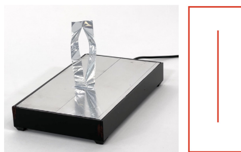
Figure 7: A slit in the film creates two parallel regions which repel to form a loop upon application of electrostatic charge.
