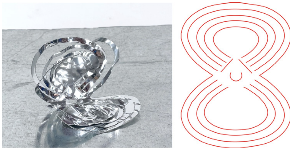
Figure 13: This clam example uses nested flaps to create a contoured shell.
