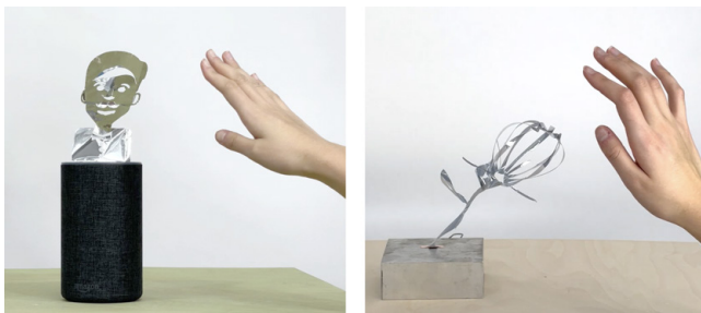
Figure 25: Users’ hand create an electrostatic attraction with inflated designs, which lean toward the user.
