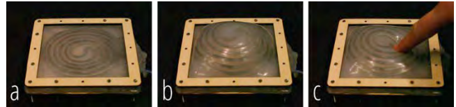
Figure 17: The resistance of liquid metal sensor changes in response to the deformation of the elastomeric channels through either air actuation (b) or direct manipulation (c).
