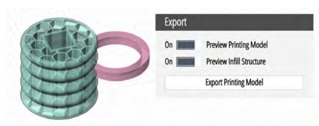
Figure 11: The interface of step 4. The software allows the user to roughly combine the attachment to the existing object, automatically stretching the adapter and generating the infill structure.
