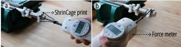
Figure 17: Setup for testing grip strength. We measure the minimum pulling force (a) and torque (b) that are required to move the ShrinCage print from a metal rod by pulling in two directions.
