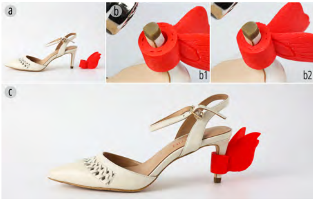
Figure 12: Example of using ShrinCage to create high-heeled shoe decoration. (a) The existing object and the print (b) are combined and shrink-fit by a heat gun. (c) The final result of the accessorized object.
