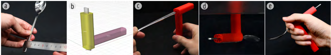
Figure 1: The ShrinCage workflow. User can (a) measure an existing object roughly, (b) design an adaptation in the software, (c) attach the printed part onto the object, (d) trigger them to be fixed in hot water, and (e) get a new functional object.
