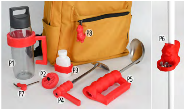
Figure 18: Outputs from the user study session: a handle for a water bottle (P1), a spinning top modified from a pen cap (P2), a pill bottle pendant (P3), a handle for a ladle that can change the direction of picking and prevent scalding (P4), a handle of a cooking spoon (P5), a key tray on the studio pole (P6), an Allen Wrench attachment for easier rotation (P7), a decorative zipper pendant (P8).
