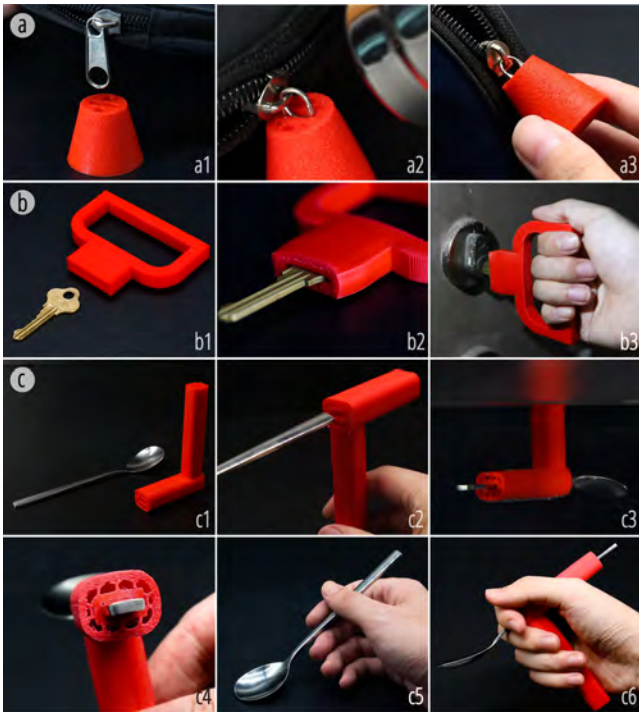
Figure 13: Design examples of ShrinCage for assistive technology. (a1) A zipper attachment, triggered by a heat gun (a2) for easier grasp (a3); (b1) a key is tightly bounded by the attachment (b2) for easier grasp (b3); (c) an attachment added to a spoon, triggered in a hot water bath (c3), can change the grasping gesture (c5-6).
