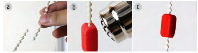
Figure 14: Attaching a ShrinCage adapter to repair a broken curtain rope.
