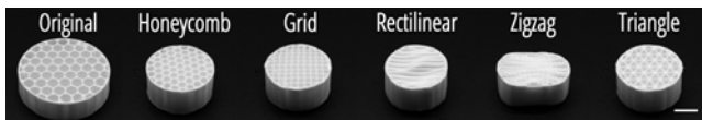
Figure 5: The shrinking test results of five different infill structures. (Scale bar: 1 cm)
