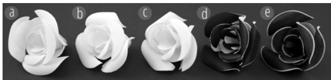
Figure 18. Five roses printed by Thermorph show a good reproducibility. Triggering temperature was 70°C, heating duration was 15 seconds.
