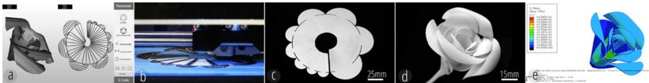
Figure 1. Thermorph overview. (a) Design editor to define and simulate the self-folding composite; (b) the printing toolpath of a flat sheet is generated from (a) and printed on an FDM printer; (c) the printed flat sheet; (d) the flat sheet self-folds sequentially into a rose; (e) finite element based simulation of the self-folding rose to verify our hypothesis on the material mechanism.
