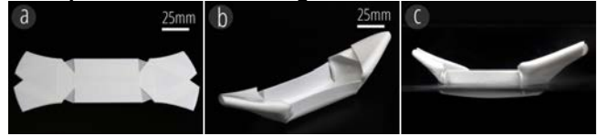
Figure 15. Self-folding boat: (a) a printed flat sheet (17.1x7.4cm); (b) a self-folded boat in 3D; (c) the boat can self-fold and float on a hot water surface.
