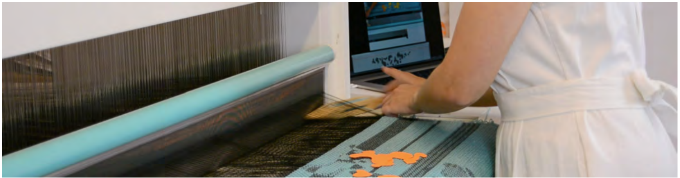
Figure 1. A system for composing fabric patterns in real weaving time on a computer-controlled Jacquard loom.
